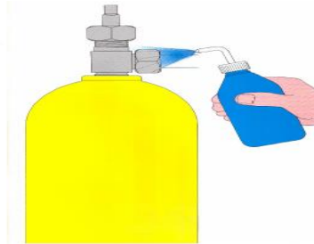
Figure 12: Method for Detecting Chlorine Leakage Using Ammonia Vapor
