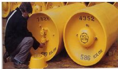
Figure 11: Store Ton Containers Horizontally with the Valve Guard Cap in its Place
